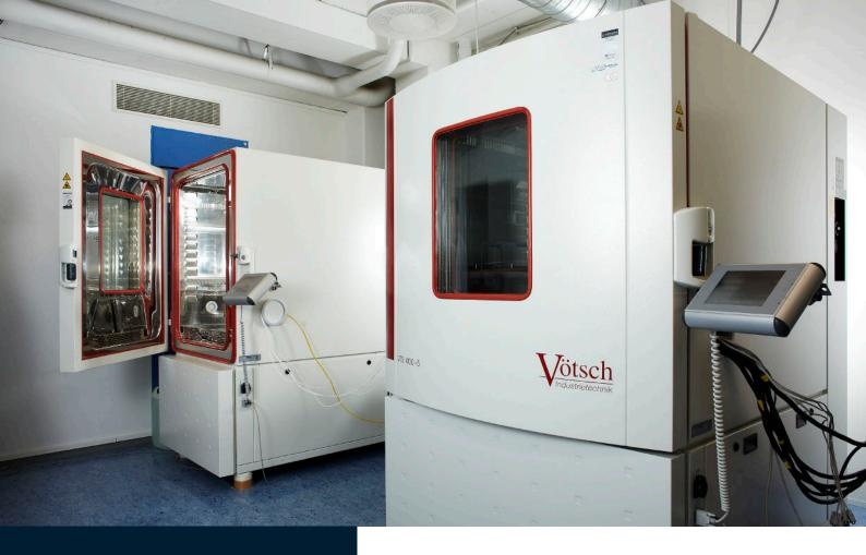
Vötsch VC-4060 climatic chamber with temperature and humidity control.
